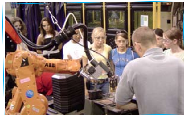
An Edison Welding Institute engineer explains the operation of a gas metal arc welding robot equipped with a laser sensor for accuracy.
